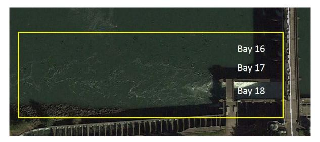
**Type of outage required** – Spillway bay gates 2-18 will need to be placed on sill (closed) with gate 1 at 0.5' opening. Fish valves 4-3 and 4-4 will be closed but not tagged out.
